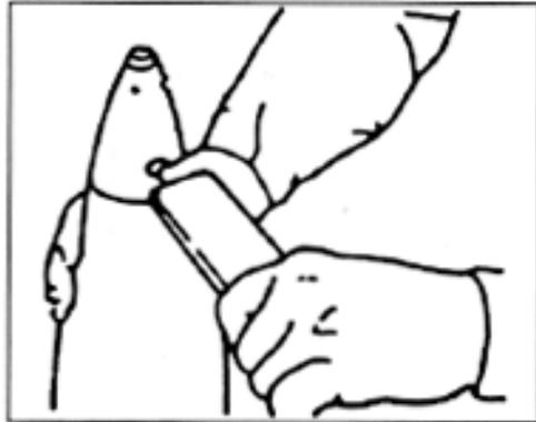
Figure 3-20. Using the M18 fuze wrench
