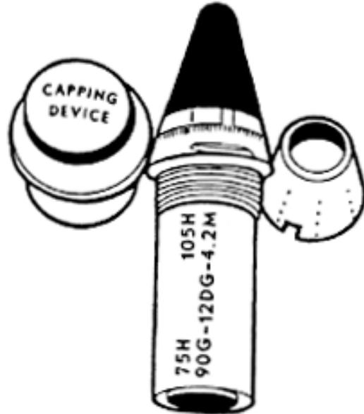
**Figure 3-27. Capping device, M513 VT fuze, M5 desensitizing cap**
